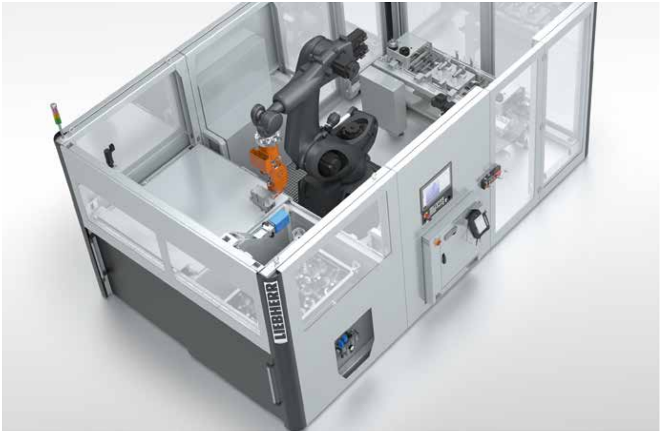
The bin picking cell
