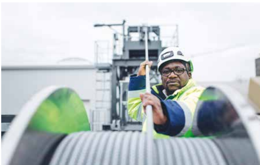
The rope is extremely light but nevertheless very strong, it has the same load capacity as a steel rope and spools up excellently
