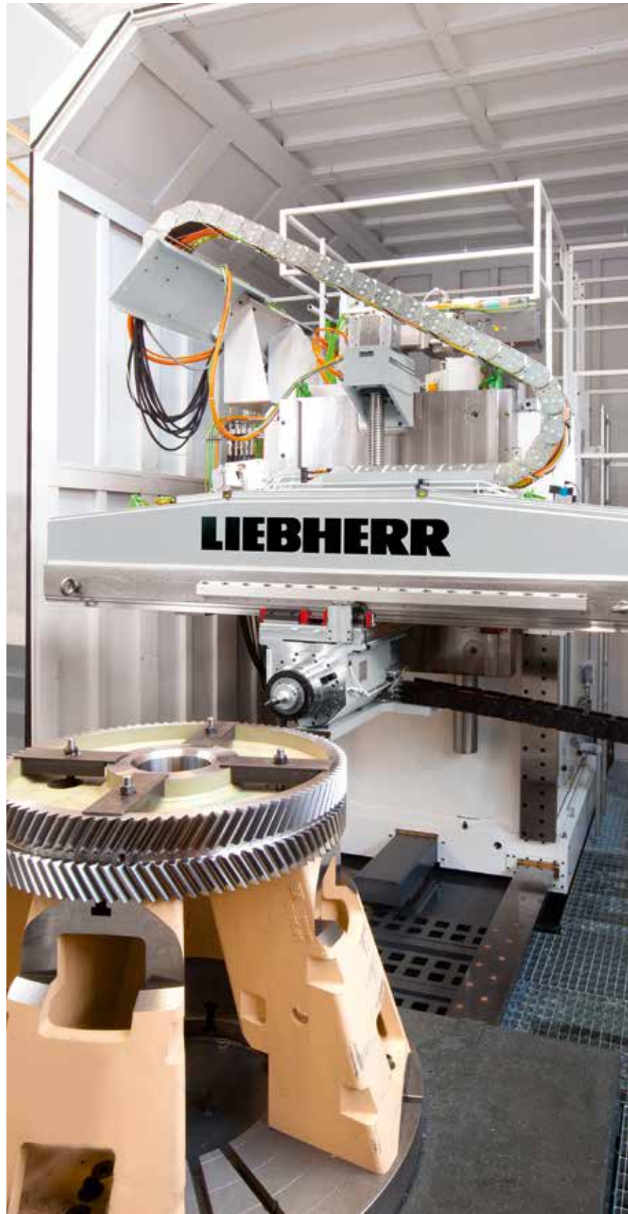
New Liebherr technology: Finger milling
