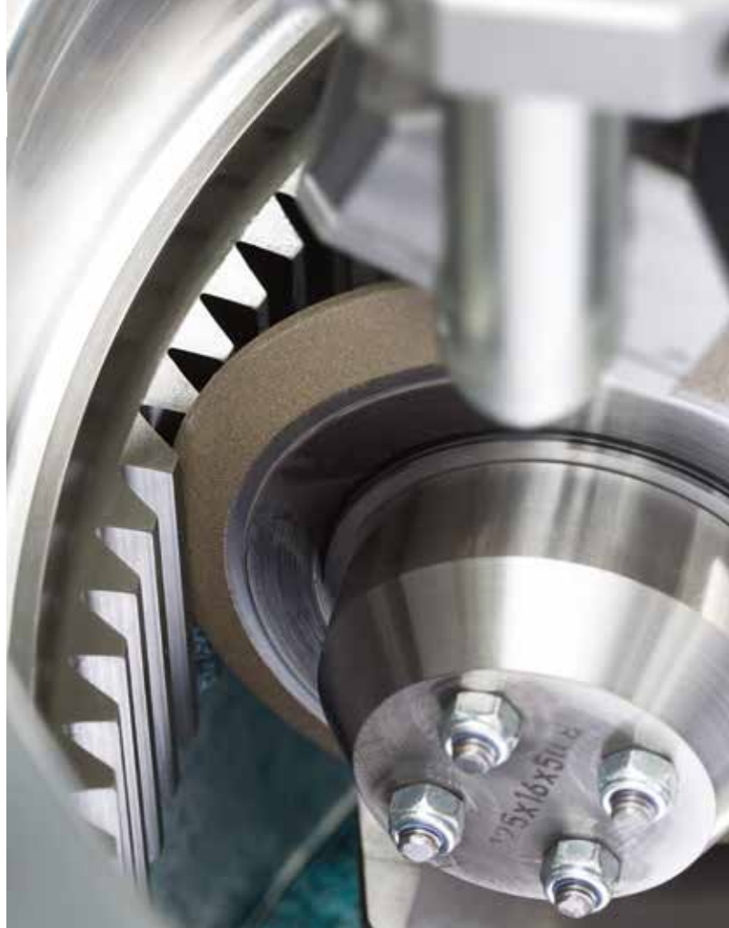
The new grinding head with CBN grinding disk
