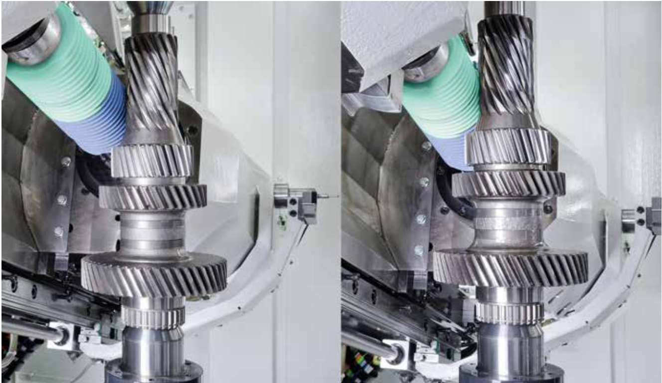
Grinding and polishing of a collision-critical gear teeth
