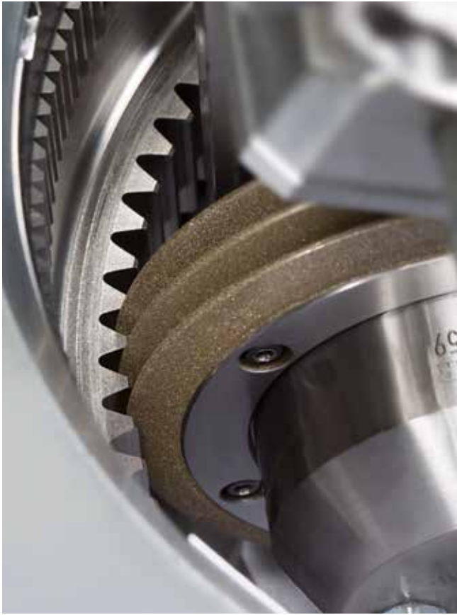
Triple-ribbed CBN profile grinding disk set from Liebherr
