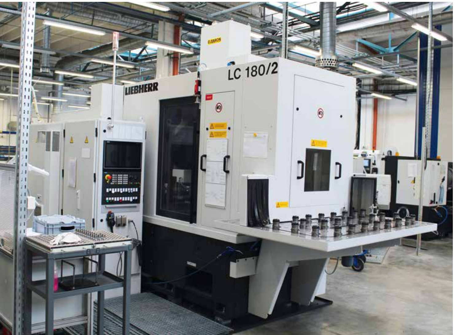
Two gear hobbing machines type LC 180 produce worm wheels, gearwheels and shafts.
