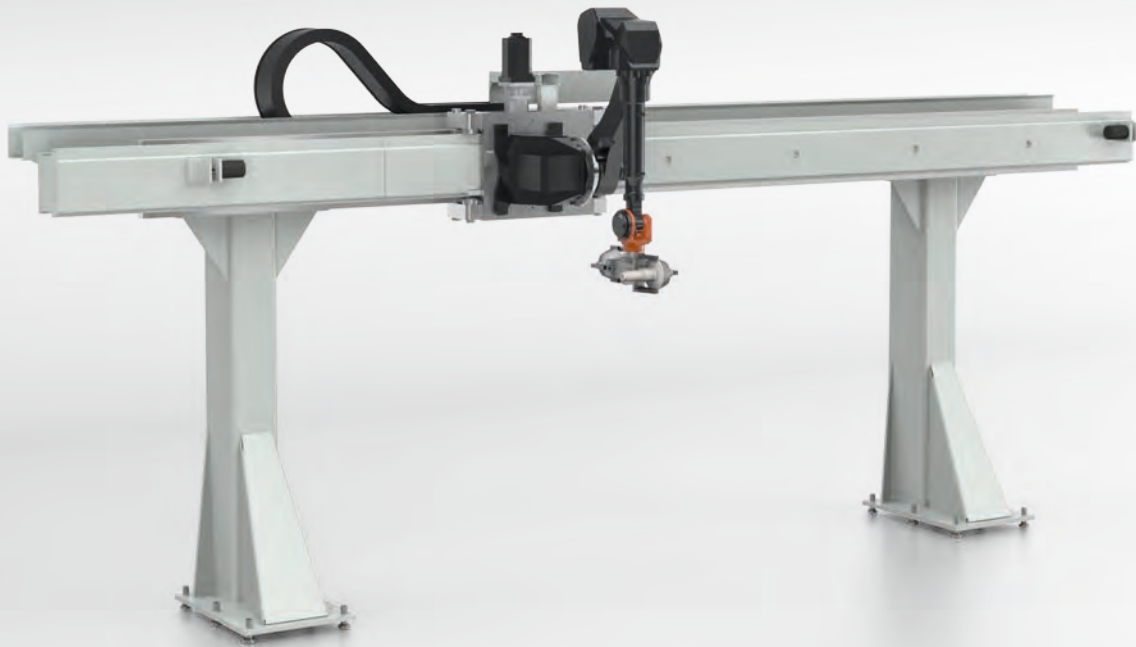
Flying robot (articulated robot at gantry)
