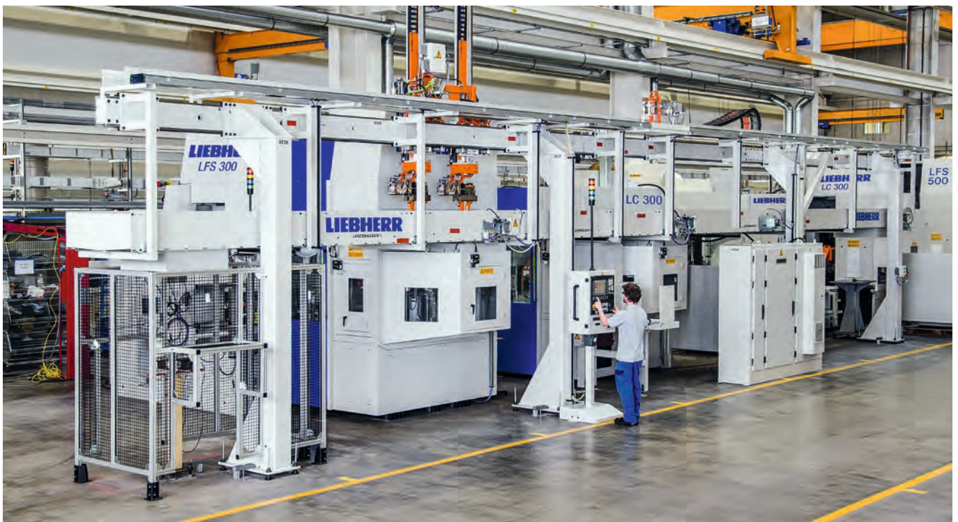
Liebherr gear cutting machines with gantry robot automation
