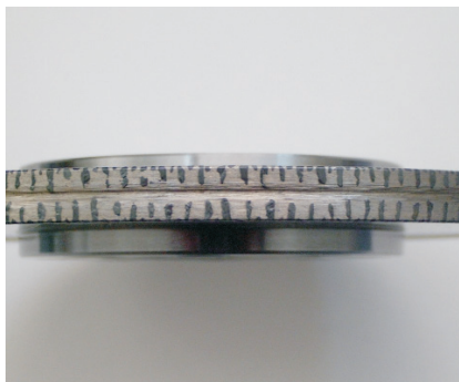
用於 Gleason-Pfauter 研磨設備的天然鑽石修砂器 - 鑽石層 = 拉長晶粒 Diamond dressing roll in natural diamond for Gleason-Pfauter grinding machines Diamond layer=elongated longs
