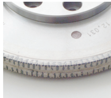
用於 Gleason-Pfauter 研磨設備的天然鑽石修砂器 - 鑽石層 = 拉長晶粒 Diamond dressing roll in natural diamond for Gleason-Pfauter grinding machines Diamond layer=elongated longs
